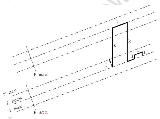
Figure D.1—Test Procedure for Pressure Temperature Cycle
