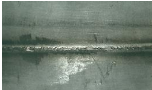
Figure C.1—Acceptable - Very good result, no discoloration
