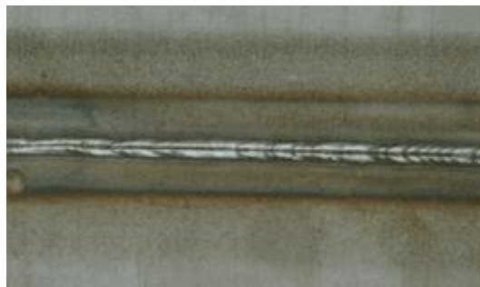
Figure C.2—Acceptable - Slight discoloration, weld shiny, no scale present
