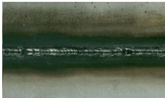
Figure C.6—Unacceptable - Very heavy oxide layer present
