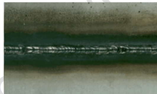
Figure C.6 - Unacceptable - Very heavy oxide layer present
