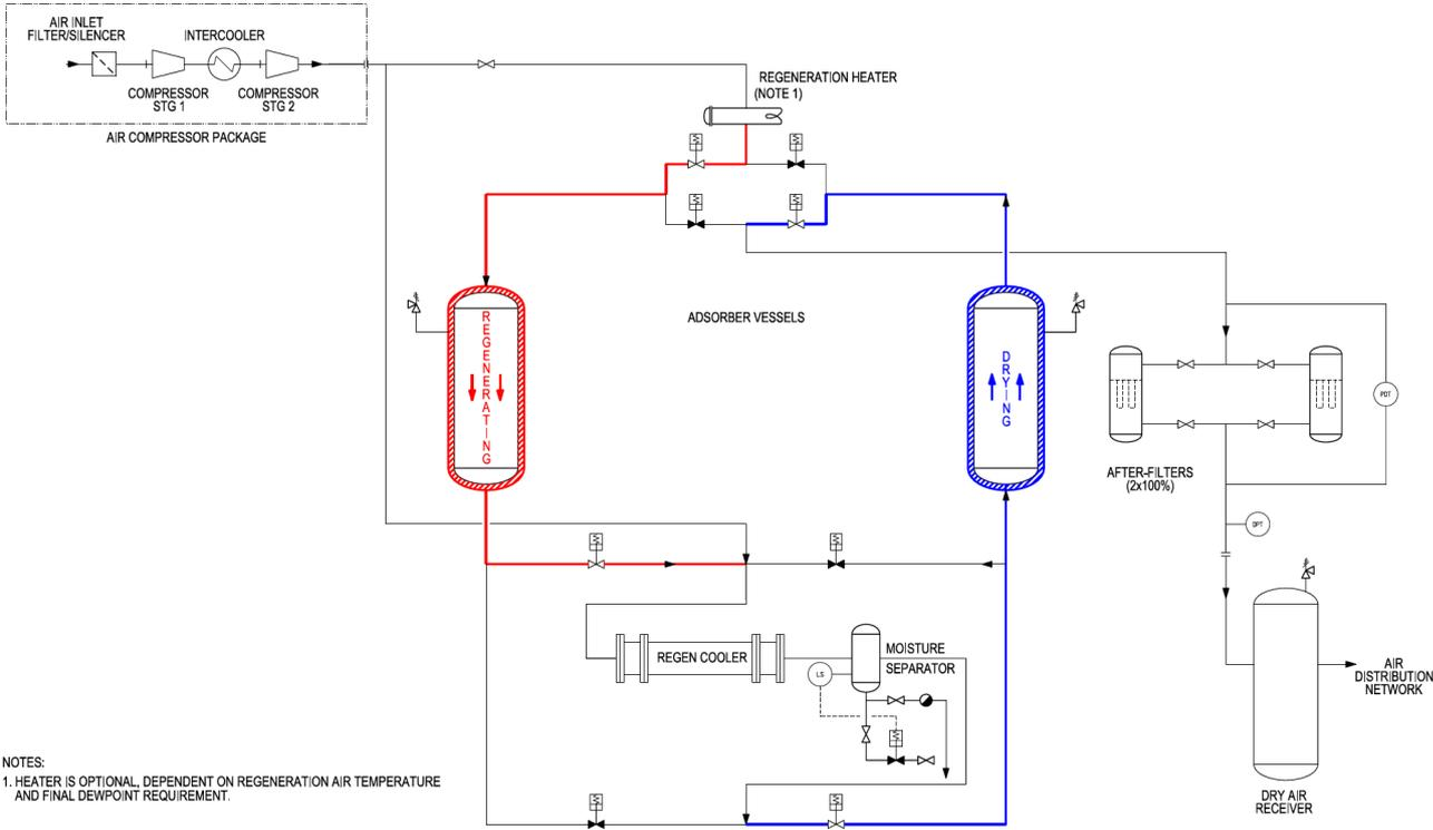
Figure B.4 – Desiccant dryer – heat of compression
