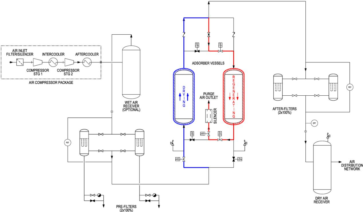
Figure B.1 – Desiccant dryer – heatless
