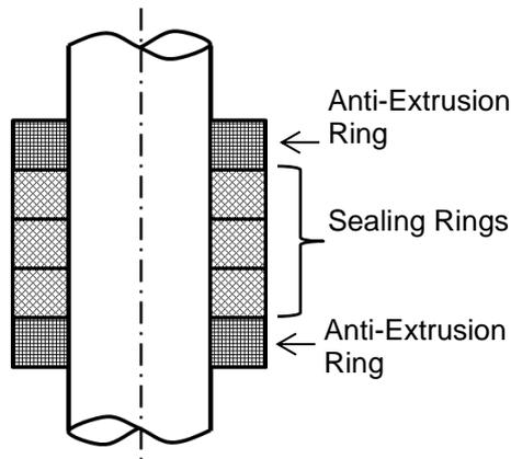
**Figure 4 – Die-Formed Flexible Graphite Packing**
