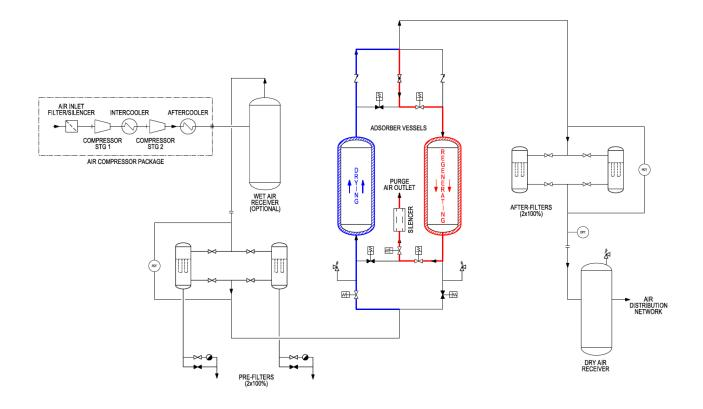
Figure B.1 – Desiccant dryer – heatless
