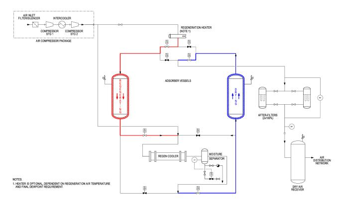
Figure B.4 – Desiccant dryer – heat of compression
