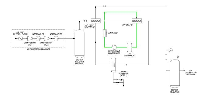
NOTES: 1. WATER SEPARATOR CAN BE INTEGRATED WITH EVAPORATOR.
